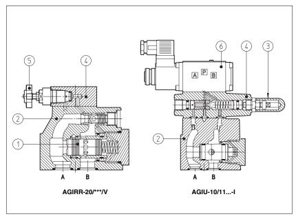
AGIR, AGIS and AGIU are double stage pressure control valves with balanced poppet designed to operate in oil hydraulic systems.
