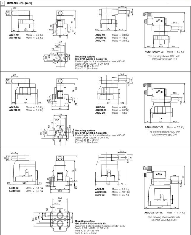
Overall dimensions refer to valves with connectors type SP-666
