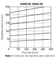
5 OPERATING DIAGRAM based on mineral oil ISO VG 46 at 50°C
