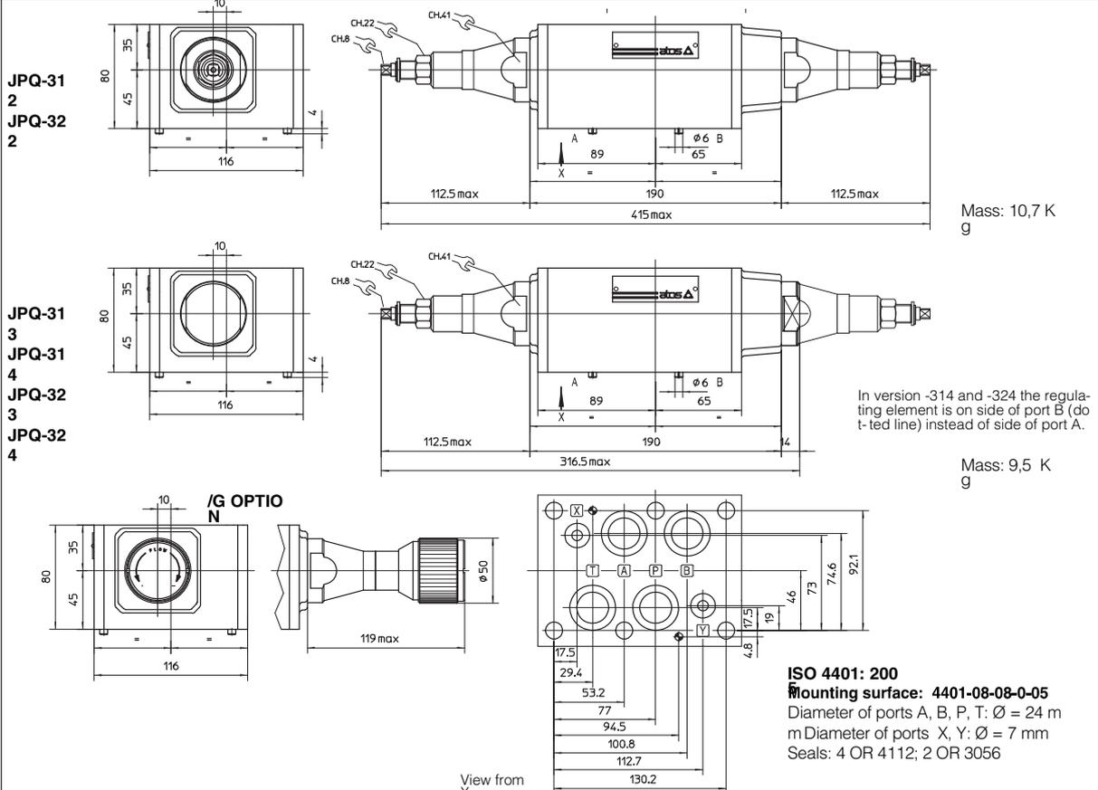
Fastening bolts: n° 6 socket head screws M12. The length depends on number and type of modular elements associated.
