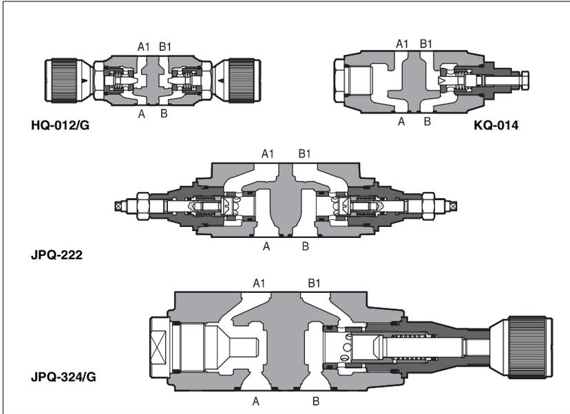
HQ, KQ and JPQ are flow throttling valves, not compensated, and with check valve in the opposite direction.
