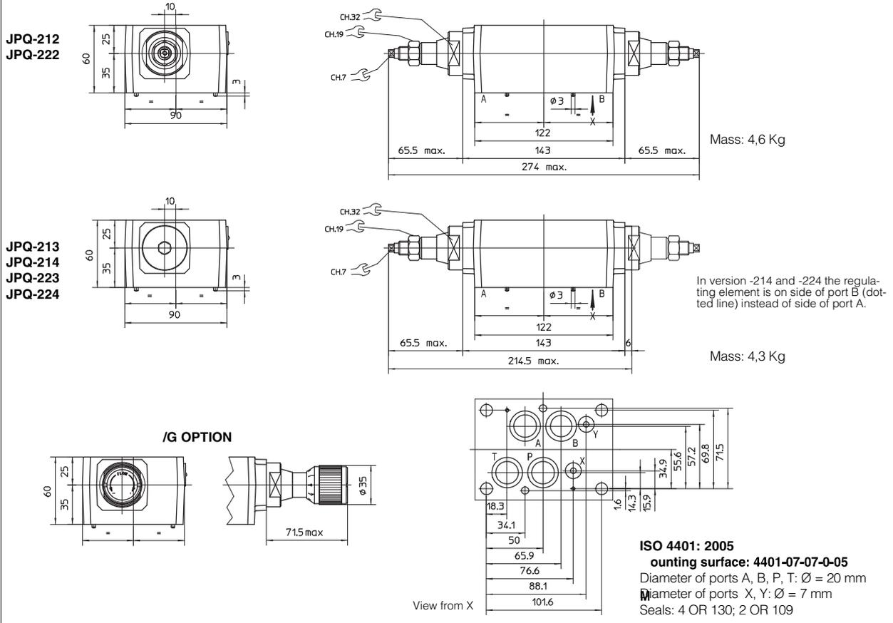
Fastening bolts: n° 4 socket head screws M10 and n° 2 M6. The length depends on number and type of modular elements associated.
