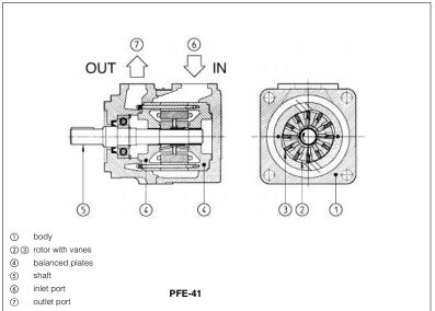
PFE are fixed displacement-twelvevane pumps, ② ③ cartridge design with integral hydraulic balancing 4 for high pressure operation and long service life with low noise level.
