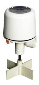
**DESCRIPTION** The Roto-Bin-Dicator® is the most universal of all level sensing technologies and is the most popular level switch used in dry bulk materials. The Roto-Bin-Dicator® is a rotating paddle type, bulk material level sensor offered with a wide variety of paddle options for unequaled application versatility. It is easy to install and requires no special tools or calibration.
