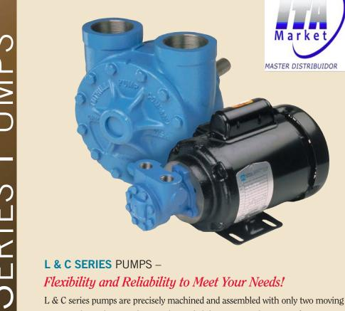
L & C series pumps are precisely machined and assembled with only two moving parts, so they achieve and retain their reliability over a wider range of viscosities than alternative pump designs. They are also available with Tuthill's unique reversing feature, as well as mounting, driving and sealing options to suit all your applications.
