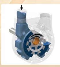
The liquid fills the spaces between the idler and rotor teeth and is carried past the crescent partition through the pressure side of the pump.
