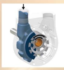
As the pump starts, the teeth come out of mesh, increasing the volume. This creates a partial vacuum, drawing the liquid into the pump through the suction port.
