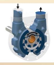
When the teeth mesh on the pressure side, the liquid is forced from the spaces and out through the discharge port.
